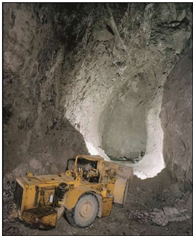
Figure 16. A large stope in Milldam Mine, worked 'in vein' before slits were used to reach the stopes(photo: Paul Deakin).
