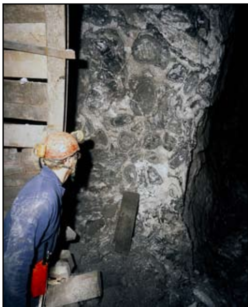
Figure 14. A cross-cut slit into an open stope in Milldam Mine, with brecciated fluorite in the stope wall (photo: Paul Deakin).
